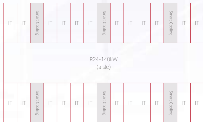
R24 Typical Layout of Dual-Row (Smart Busway)
